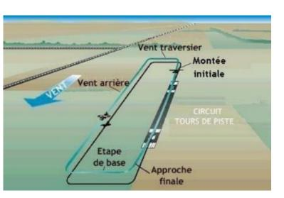
The traffic pattern, also called aerodrome circuit, is a maneuver that airplane makes around the runway, at a height of 1000 feet.
